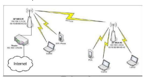
As you have previously set up your NanoStation5 as a AP, you are now able to set up an other device as a repeater.
